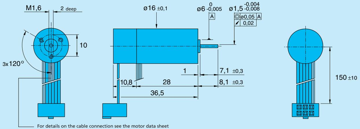
**Brushless DC-Servomotor 2036 U ... B with Encoder IE2 – 512**
