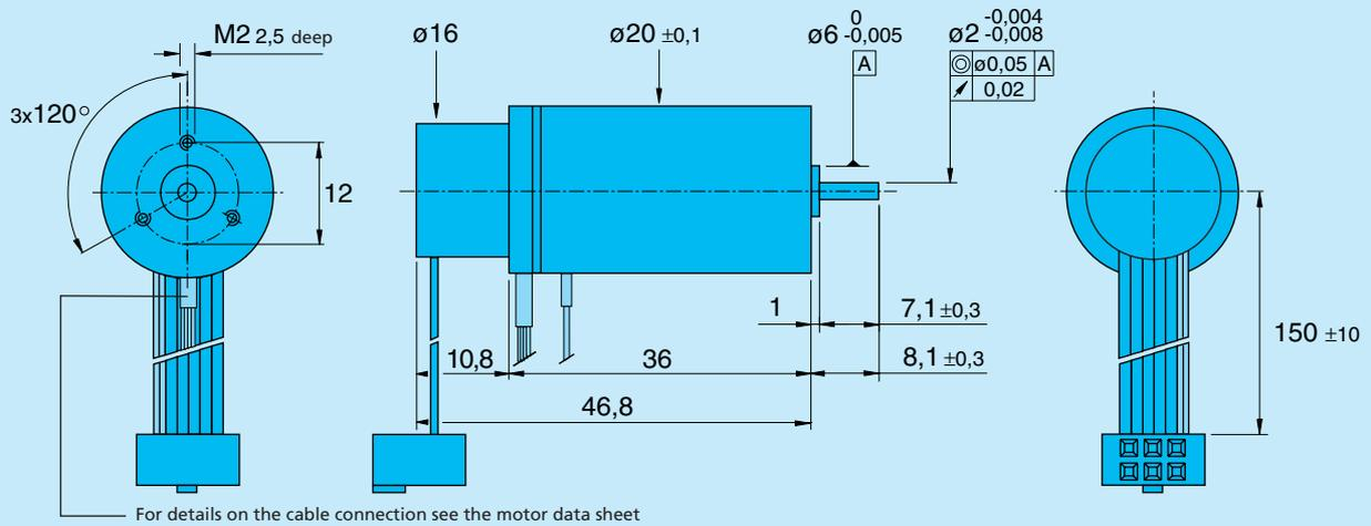
**Brushless DC-Servomotor 2444 S ... B with Encoder IE2 – 512**
