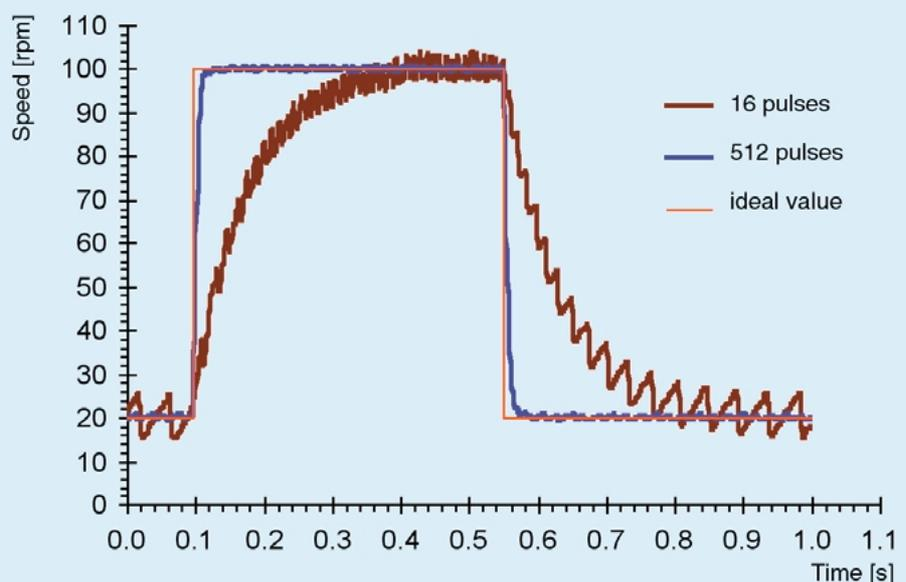
Figure 4: comparison of two encoders with speed control
