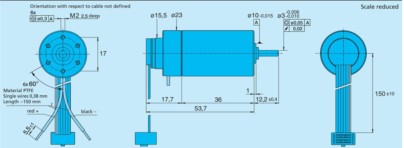
**Brushless DC-Servomotor 1628 T ... B with Encoder IE2 – 512**
