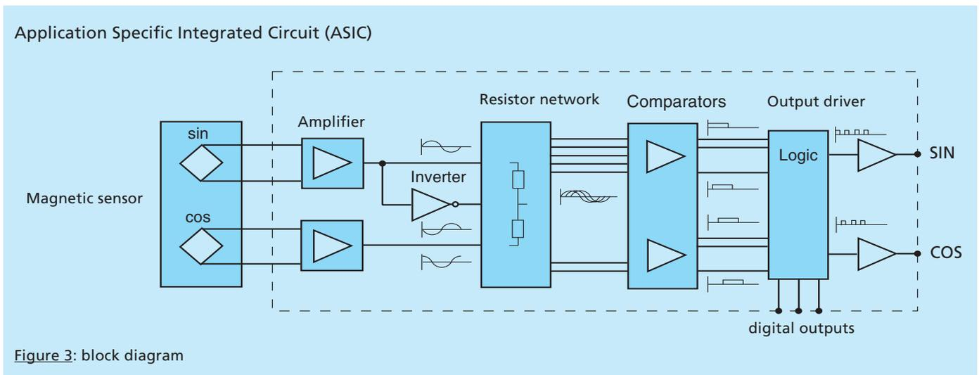
Figure 3: block diagram
